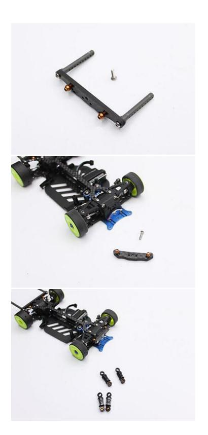
Assemble your shock towers as the images show. Use some M2x4 BH to attach the threaded balls to both front and rear towers.
