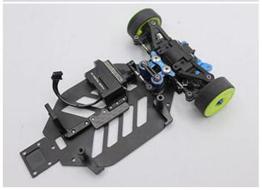
The servo mount is designed to be used with a smaller servo such as the RRE007. This servo is more than strong enough (actually has more torque than the larger ones) to handle the job and it lowers the CG and balances the car better.
