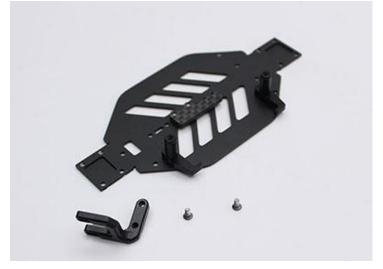
First we will start by mounting the battery holding hooks. Use the long M2x8 CS screws and thread through the bottom into the post. The pin that goes into the chassis could be a little tight. You could drill this out slightly if you want, but usually tightening it down will ensure the hooks don't move. You can use shims here to space the posts up if your battery is taller.
