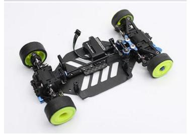
Now install the driveshaft. Be careful in this step! The driveshaft is made from 7075 aluminum, but it is still very long and skinny. It can bend if you are not cautious. If you don't want to risk it, remove the front steering, and access the gears on both front and rear through the shaft bearing top covers.
